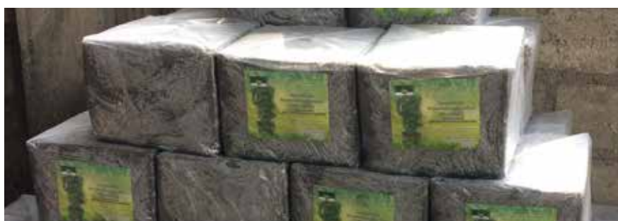
A mix of naturally available materials with dimensions 10” x10” x 10” & 12 kg weight
